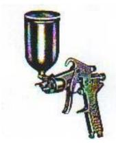
Here is a better choice, a "gravity feed" gun. These are usually smaller in size, intended for holding only a small quantity of paint (about 500 mL maximum), easy to wash out, ideal for our purpose. Sometimes the feed cup is mounted vertically above the gun (not so good). Sometimes the feed cup is offset to the side, as in the illustration. Either way, fluid drains into the gun by gravity, not pulled up by suction. For our purposes, **the gravity-feed gun is the only way to go.**
