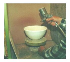
we shake up the glaze bottle, measure out 50 mL, and spray it all evenly inside while the bowl rotates on the turntable.
