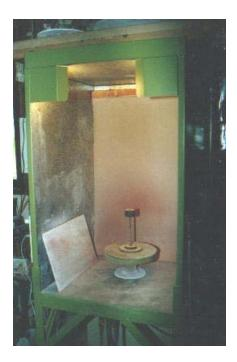
Often the bottom of the pot will be smaller than the size of your turntable, so you'll need some kind of pedestal to stand the pot up higher. This is so that you can spray adequately right down to the bottom edge of your pot, without the top of the turntable getting drowned in glaze too. You'll find use for a variety of pedestal shapes, beginning with something as simple as a jam jar. Tall and short, wide and narrow.
