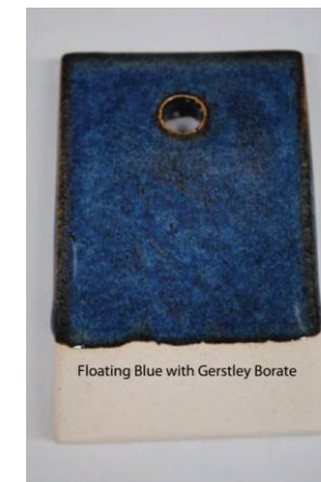
Gerstley borate used in glaze formula. Floating Blue (left) and PV Variegated Blue (right)
